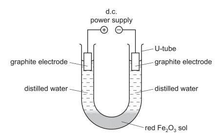
(b) The student placed a few cm<sup>3</sup> of the sol at the bottom of the U-tube and poured 10 cm<sup>3</sup> of distilled water into each side of the U-tube, without disturbing the sol. The two layers of distilled water were colourless at the beginning of the experiment. Graphite electrodes were inserted and a current was passed. After 30 minutes a difference was noted between the distilled water in the two sides of the U-tube.
